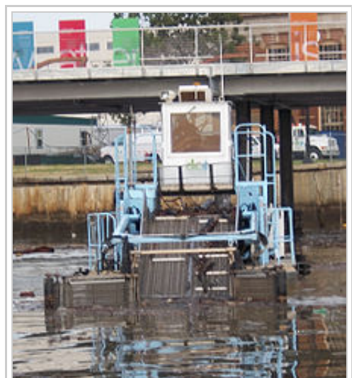
Skimmer boat used to remove floating debris and trash from the Potomac and Anacostia rivers
